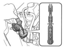
If any washer doesn't work, the washer fluid reservoir may be empty. Please check the fluid level on the level gauge. If the fluid level is near LOW level, add washer fluid.
