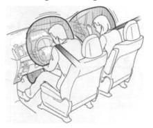
The frontal airbags, including the driver's airbag and front passenger airbag, are designed to inflate in moderate to severe frontal or near-frontal collisions, protecting the head and chest of the driver and front passenger from striking interior objects such as the steering wheel or a window
