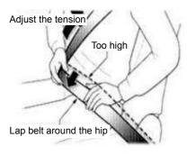
Arrange the lap belt around the hip rather than the waist, and then pull the shoulder belt upward to a proper position.
