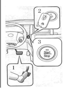
If you cannot get into the vehicle or start the engine with the card key, the battery may have depleted. Please replace the battery following the instructions in "Replace Battery in Card Key" in this chapter.
