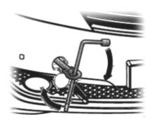
Tighten the front tow hook with the wheel nut wrench.
