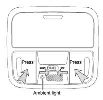
The front interior light is operated with a 2-position slide switch:
