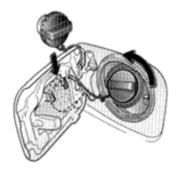
To remove the fuel tank cap, slowly rotate it anti-clockwise, wait for a moment and then remove it. Hang the cap on the support after removing it.
