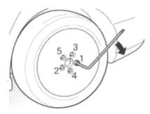
Lower the vehicle completely and tighten the wheel nuts.
