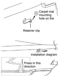
Press down the retainer clips in the direction shown in the figure above, make sure the clips are locked in place, and then install the carpet mat.
