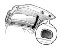
To close the rear door, pull it down and then firmly press it. Make sure to pull it upwards to check whether it is locked firmly.
