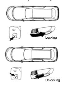
To lock/unlock all doors, press the switch on the smart key slowly and firmly.
