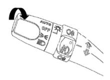
The rotation switches (AUTO, OFF, 300; and ≡□) on the lever controls the width-indicator lights and headlights.
