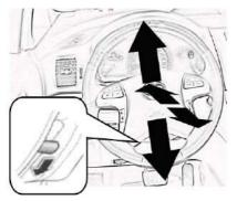
To change the steering wheel angle, hold the steering wheel, press down the steering wheel adjusting handle and adjust the steel wheel to desired angle. Release the adjusting handle to allow the lever to return to the lock position.
