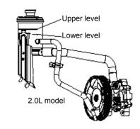
Check the power steering fluid level at least once a year. To check the fluid level, the vehicle must be on level ground and the engine must be cold. The fluid level must fall between the UPPER LEVEL and LOWER LEVEL marks on the reservoir. If the fluid level is below the LOWER LEVEL, add the specified power steering fluid to the UPPER LEVEL.
