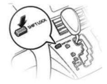
If you cannot shift the selector lever out of P position even if the brake pedal is pressed down, use the Shift Lock button as follows:
