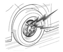
Disc bake pads have built-in wear warning indicators that make warning sound when the worn brake pads must be replaced by new pads.
