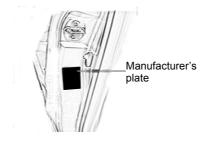
VIN is also printed on the manufacturer's plate at the bottom of the right side wall B-pillar, as shown in the figure above.
