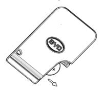
3. Insert a new battery and then the mechanical key into the card key.
