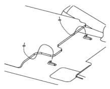
Carpet mat and carpet mat retainer clips are supplies in the standard configuration. The carpet mat is fastened by the retainer clips. The carpet mat retainer clips are designed to prevent the carpet mat from sliding ahead, which may interfere with the pedal operations.
