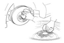
Before putting on the wheel, clean up the mounting surface with a wire brush to remove any rust or dirt. When installing a wheel, make sure the metal to metal contact on the mounting surface is good. Otherwise it may reduce the driving comfort, cause the wheel nuts to get loose and eventually cause the wheel to come off while driving.
