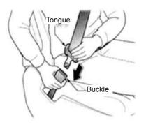
Adjust the seat to your desired position while you are sitting in the seat. To fasten the seat belt, pull out the seat belt from the retractor and insert the tongue into the buckle.
