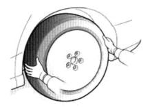
Remove the wheel nuts and change the tire.
