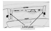
Lift up the glove box in the direction of the arrows to remove the glove box.Pay attention to the limit posts on both sides.
