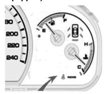
If your vehicle is equipped with seat belt warning sensors, there is a front passenger seat belt warning indicator on the combination switch, which is indicated by the black arrow in the figure above. If the front passenger seat is occupied without using the seat belt, this indicator turns to remind the front passenger to wear the seat belt. After the seat belt is fastened, the warning indicator goes off. When the front passenger seat is not occupied, the warning indicator remains off.
