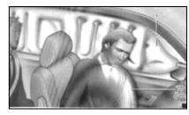
Curtain airbags, if equipped, drop down from the roof along both sides of the cabin in moderate to severe side collisions to give better protection.
