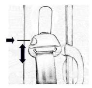
Adjust the shoulder belt buckle to proper position.
