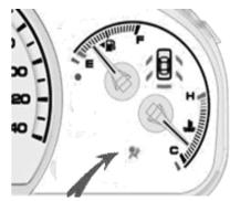
Under the control of an ECU which features self-diagnostic capability, the state of the SRS airbag system is indicated by a warning indicator on the instrument panel.
