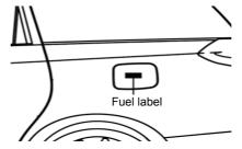
Fuel label is pasted on the inner side of the fuel filler cap, as shown in the figure above.
