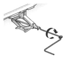
Make sure no one is in the vehicle, and then raise it high enough to remove and change the flat tire.
