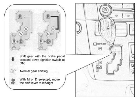
The automatic transmission is equipped with a shift lock system to minimize the possibility of incorrect operation. The shift lever cannot be moved out of P gear unless the brake pedal is pressed down while the ignition switch is at ON.
