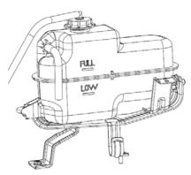
Check the coolant level in the transparent coolant reservoir when the engine is cold. The coolant level must fall between the FULL and LOW line. (Refer to the next section "Which Coolant to Use" to choose a coolant.)
