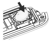
4. Install a new battery in place with the anode side (+) facing upward. Insert the mechanical key back into the electronic smart key. Firmly install the cover of the electronic smart key.
