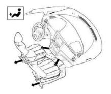
4. - This mode directs most of the air to the floor outlets and front windshield.
