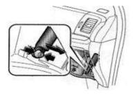
1. Open the glove box and pull off the damper, as shown in the figure above.
