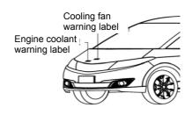
The warning labels to the cooling fan and change of engine coolant are pasted on the inside of the front compartment.
