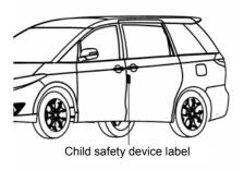
2 child safety device labels are pasted in the middle of the front surface of the sliding door metal sheet in a symmetrical pattern.
