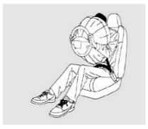
In the event of a head-on collision more severe than a certain threshold, the sensors detect that the vehicle is slowing down fast and send a signal to the controller to inflate the frontal airbags in a very short time.
