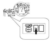
The parking assist system works if you press the switch when the Start button is at ON, and the shift lever is at P or any gear other than Neutral.
