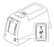
Press the seat heater switch to heat up the driver's seat which is equipped with a heater.
