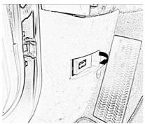
Pull the engine hood release handle and the hood will pop up slightly.
