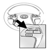
There are 3 buttons on the left of the steering wheel hub for setting the sound system. You can operate the basic functions of the sound system without getting your hands away from the steering wheel.
