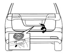
To open the rear door, first unlock it with the mechanical key or lockout device, and then pull the rear door handle upward.
