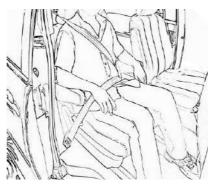
To fasten the seat belt when an outer armrest is used, arrange the shoulder belt above the armrest and the lap belt under the armrest.
