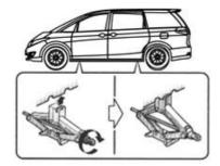
Position the jack at the correct jack point as shown in the figure above.
