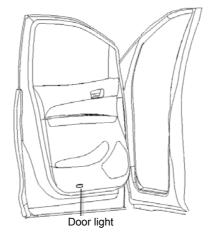
Each door has a door light. When you open a front door, its door light will turn on.
