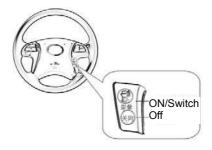
Press the Vision ON/Switch button on the steering wheel to enable the front right vision.
