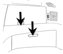
Press the button to open the top right glove box, and press the cover downward to close it.
