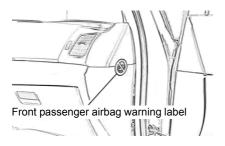
The front passenger airbag label is located on the right side of the instrument panel.
