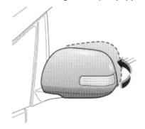
To park the vehicle in narrow space, fold the rearview mirrors backward to prevent damage.
