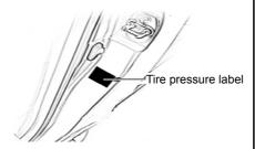
Tire pressure label is located near the bottom of the left B-pillar.
