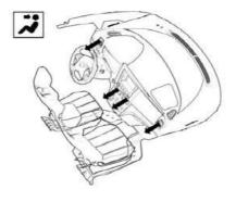
2. This mode directs half of the air to the instrument panel outlets and the remaining air to the floor outlets.
