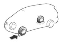
When jacking up the vehicle, block the wheel diagonally opposite to the flat tire to keep the vehicle from rolling.
