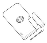
Using the Mechanical Key in the Card Key
