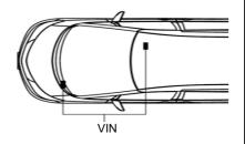
Two VIN plates on this vehicle are respectively located on the top left side of the instrument panel and on the floor crossmember under the front passenger seat, as shown in the figure above. VIN is a unique serial number used for registration of the vehicle owner.
