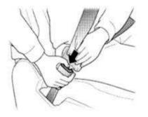
To release the seat belt, press the buckle release button and let the belt retract.
