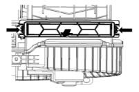
3. Press the latches on both sides to release them, and then pull out the filter.
