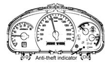
4. Make sure the indicator is flashing before leaving the vehicle.
