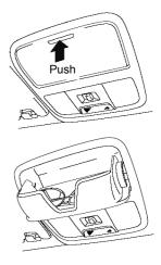
To open the sunglasses bracket, press it at the front edge. To close the sunglasses bracket, push it until it is locked in place.
