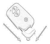
Press the release switch downwards and then remove the mechanical key.
