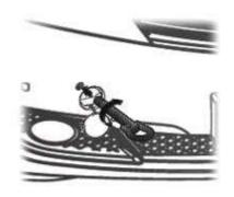
Get the front tow hook on hand. Install the front tow hook into the hole on the front bumper by rotating it clockwise (see "If You Have a Flat Tire" for the storage location of the toolkit).
