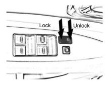
Both front doors are equipped with a power door lock switch. These two switches can lock/unlock all side doors.
