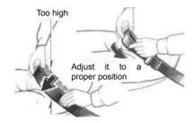
Adjust the seat belt to around the hip and retract the excessive length.
