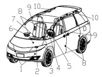
The major components and their locations of the M6 SRS airbag system are shown in the figure above.
