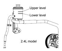
The fluid level may drop if there is a leak in the system. In this case, regularly check the fluid level and have the system inspected and repaired.
