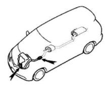
Three-way catalytic converter is a device installed in the exhaust system to control emissions.
