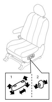
1. Regulating switch of seat height, position and cushion angle
