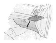
The filter is installed behind the glove box.
