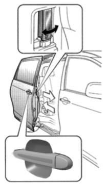
Open: pull the door handle outwards to unlock it and then slide it backward. Fully open the sliding door and it will be locked up by the positioning lock at the bottom.
