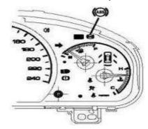
When the warning indicator stays on and the braking system indicator remains off, the ABS system, traction control system and stabilization control system are not working normally. However, the
