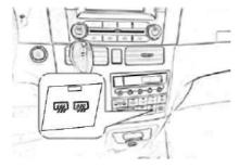
Press the button on the A/C panel to turn on/off the rear defroster.
