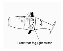
The front/rear fog light switch is located beside the headlight switch (front fog light ♣, rear fog light ♣.). When the light switch is at ♣, or ♣D, you can turn on the front fog light with this switch. When the light switch is at ♣D or when the front fog lights turned on, you can turn on the rear fog lights with this switch.
